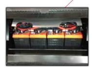
Four Group 31 batteries, electrically isolated from the truck, power the system.
