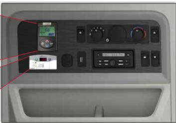
The sleeper control panel is a convenient central location for all the items you need to control the sleeper environment, along with entertainment and interior lighting.
