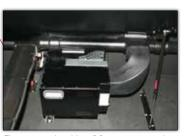
The compact brushless DC compressor and evaporator assembly is strategically located in the sleeper storage area.
