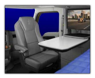
The Drviers' Studio includes the 180-degree swivel passenger seat and swivel table option set, which maximizes the driver's living space by combining the cab and sleeper into a large studio, allowing the driver to relax in comfort in the passenger seat rather than being confined only in the back of the sleeper. It also allows for viewing of the TV from the passenger seat or the bunk.
