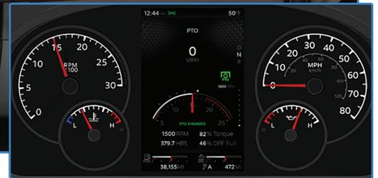
Standard Instrument Panel with 7-Inch Digital Display
